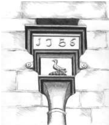
Bramley Grange, Rotherham – rainwater head, 1756. Drawn October 2018.
