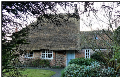
Old Thatch, Long Marston (YVBSG 0294). A double-aisled timber-framed house, perhaps constructed c1500 from re-used timbers.
