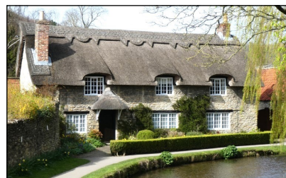
Beck Isle Cottage (YVBSG 0323). This picturesque much-photographed cruck-framed house was renovated 1938 when dormer windows were added and roof thatched with Norfolk reed. Contained a fine carved door to the C17 century spice cupboard or salt box.
