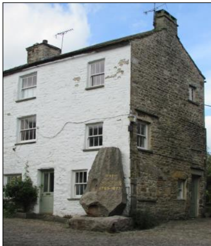
Sedgwick Cottage (YVBSG 531). The cottage is three storeys high and built with sandstone rubble with large well-worked quoin blocks. The original cottage consisted of one room on each of the three floors.
